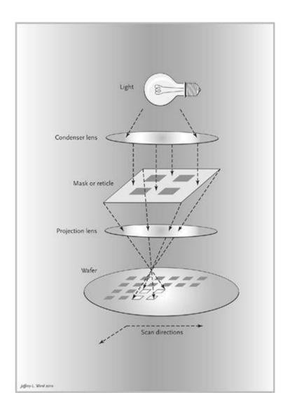
The end of Moore's law. Chips are made the same way as designs on T-shirts. Instead of spray painting over a stencil, UV light is focused on a stencil, burning an image onto layers of silicon. Acids then carve out the image, creating hundreds of millions of transistors. But there is a limit to the process when we hit the atomic scale. Will Silicon Valley become a rust belt? (photo credit 1.1)
